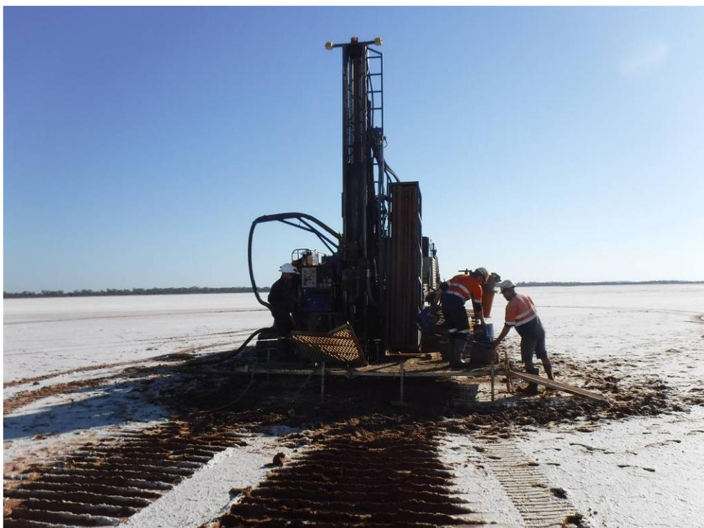
*Figure 1. Aircore rig on Lake Yindarlgooda.*
