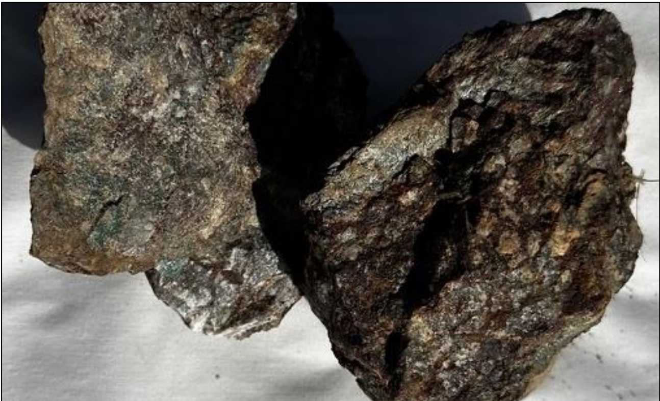
Figure 5: Lone Star Prospect sample TEM15 that assayed 4.11% Cu and 82.2 - 101 g/t Au (101 g/t Au = 3.2 Oz/t Au).
