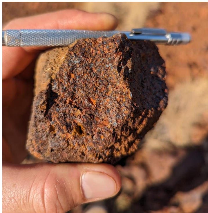
Figure 10: Robe River pisolite hand sample located from Mesa 3 (200m west of tenement boundary) showing representative Robe River pisolite found on Mesa 1 and Mesa 2
