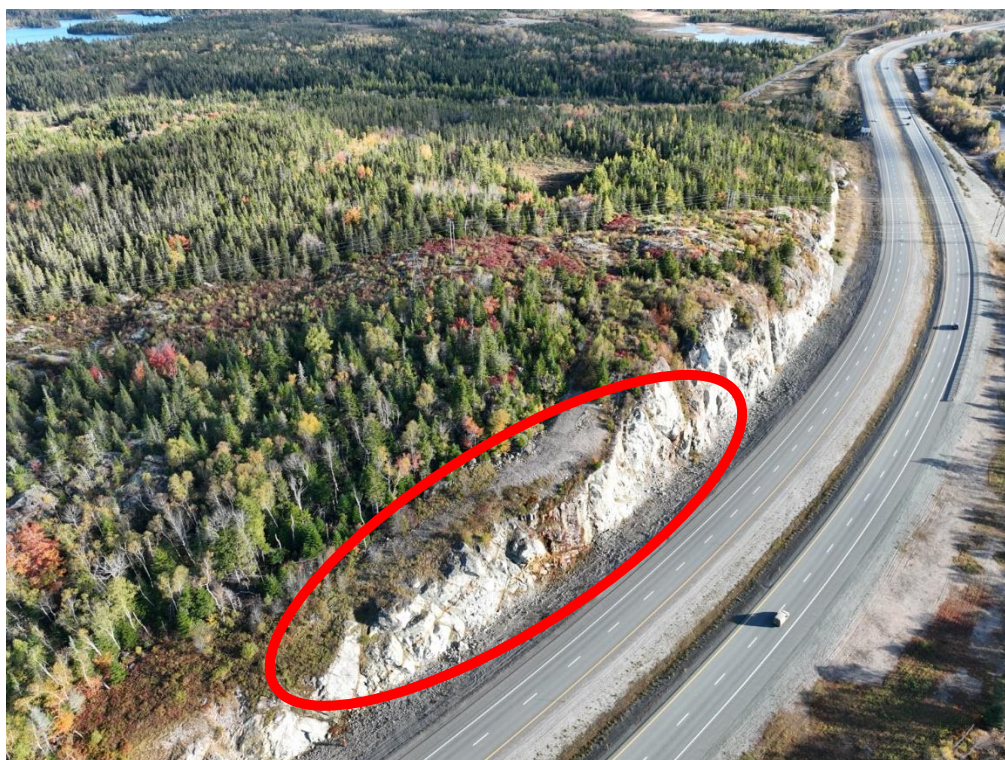
Figure 7: Prince of Wales roadside exposure with sulphide iron staining near mineralised rock chips grading up to 1.95% Sb, 3.37% Cu, and 939 g/t Ag. See Figure 6 for location.
