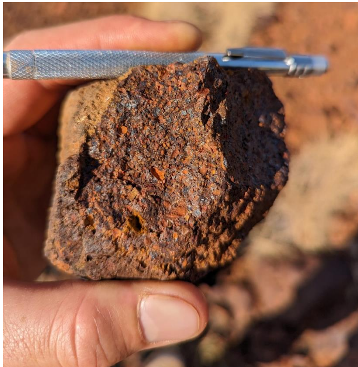
Figure 16: Robe River pisolite hand sample located from Mesa 3 (200m west of tenement boundary) showing representative Robe River pisolite found on Mesa 1 and Mesa 2
