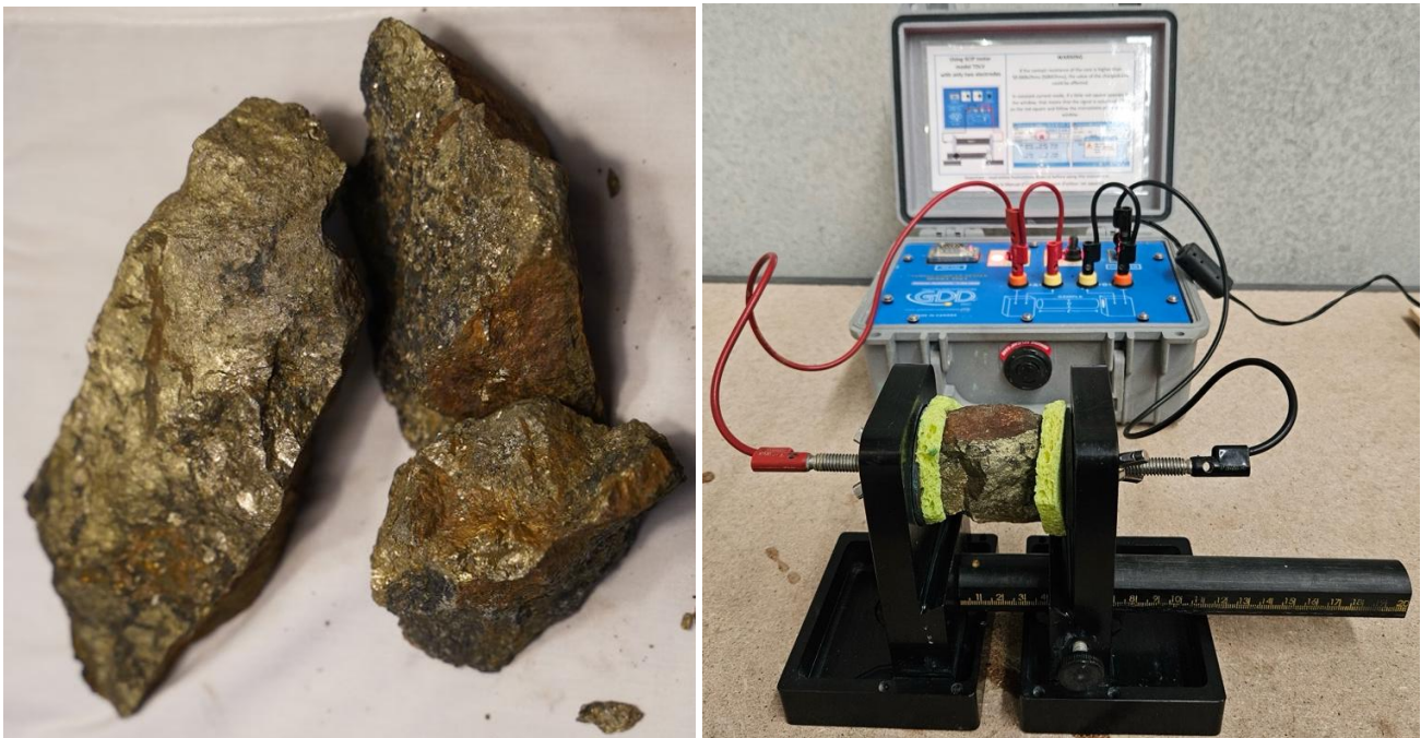
Figure 1: Prince Of Wales prospect sample RK008302 10.15% Cu and 65.8g/t Ag 2 , being tested for Induced Polarisation, chargeability, galvanic resistivity and inductive conductivity
